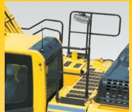
Hand rails and anti-slip plates
