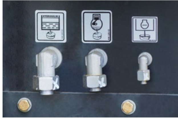
Smart: operating fluids can be drained from the outside.
