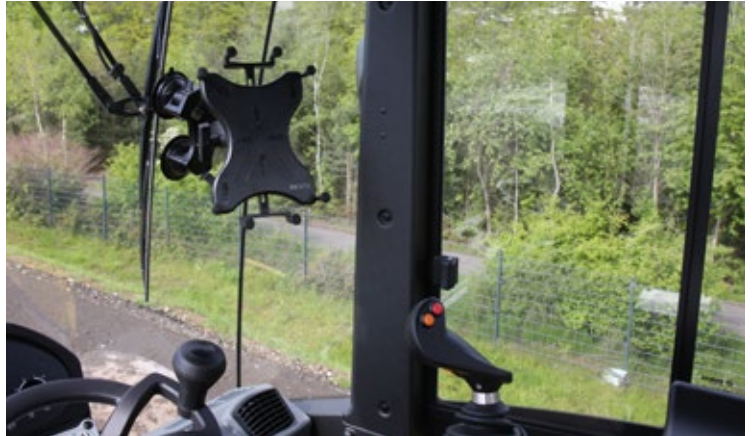
Quickly installed: the tablet holder can be conveniently placed anywhere in the cabin using the quick-release fastener.
